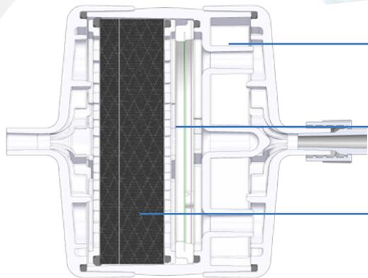
Integrated water trap to capture water vapour that carries viruses and bacteria
